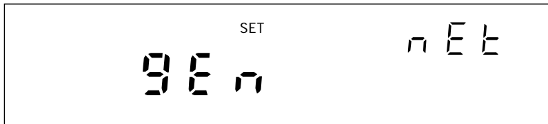
Network display for setting the network type to general
