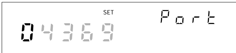
Socket Port display for setting the first digit (for the example 0 4369)
